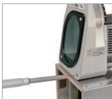
Precise adjustment of the electrode's stick-out.
