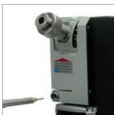
Precise adjustment of the electrode's stick-out.
